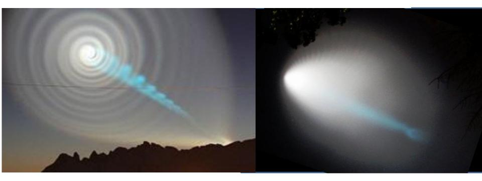
BOTH IMAGES SHARE WHITE PLUME OF MAIN ENGINE EFFLUENT AND A NARROWER BLUE PLUME POSSIBLY FROM THE HYDRAZINE-FUELLED HYDRAULIC POWER UNIT [HPU] NEEDED TO SWIVEL THE ENGINE NOZZLE [UNDER NEARLY IDENTICAL SOLAR BACKLIT ILLUMINATION CONDITIONS]. MUCH SLOWER PLUME EJECTION SPEED FROM HPU VERSUS ENGINE CREATES THE MUCH NARROWER PLUME SPREAD PATTERN AS OBSERVED.
